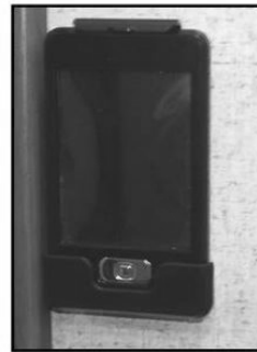
Handheld wireless remote control located at entrance door
